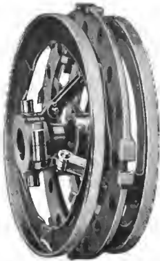
Three-Plate Disc Clutch with Cork Inserts. The Autocar Company.
